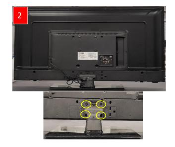
2. Middle stands are disassembled by removing four screws attaching it to TV unit as shown in figure 2
